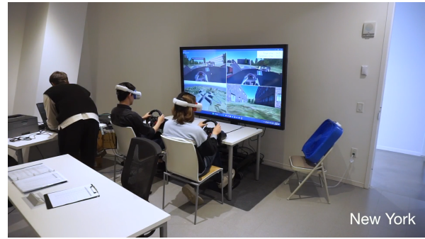
Fig. 1. The experiment was conducted in virtual driving simulators in two locations: Haifa, Israel and New York City, New York. Two participants, seated next to each other, had multiple driving interactions with each other in the same StrangeLand driving environment [20].
