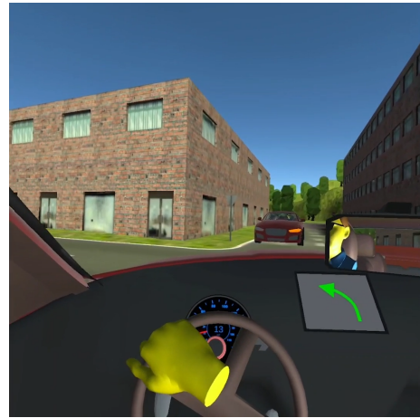
Fig. 2. Each participant’s view within the virtual environment provides a realistic driving view that consists of the dashboard of their own vehicle, their hand movements projected within the virtual environment, the simulated external environment, and the car of the other driver. The green arrow instructs the participant of the next maneuver.
